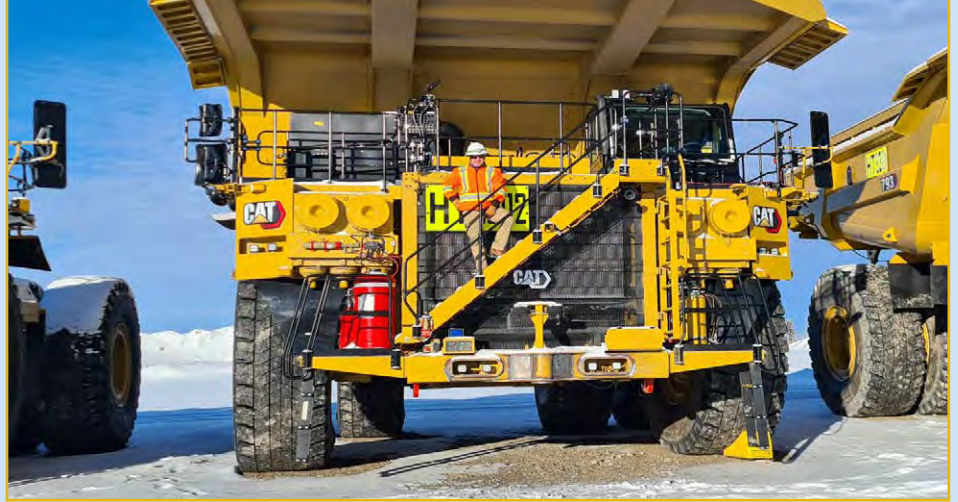
240 tonne rigid frame haul truck - January 2024
