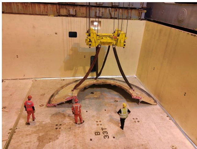
Ball mill head segment
