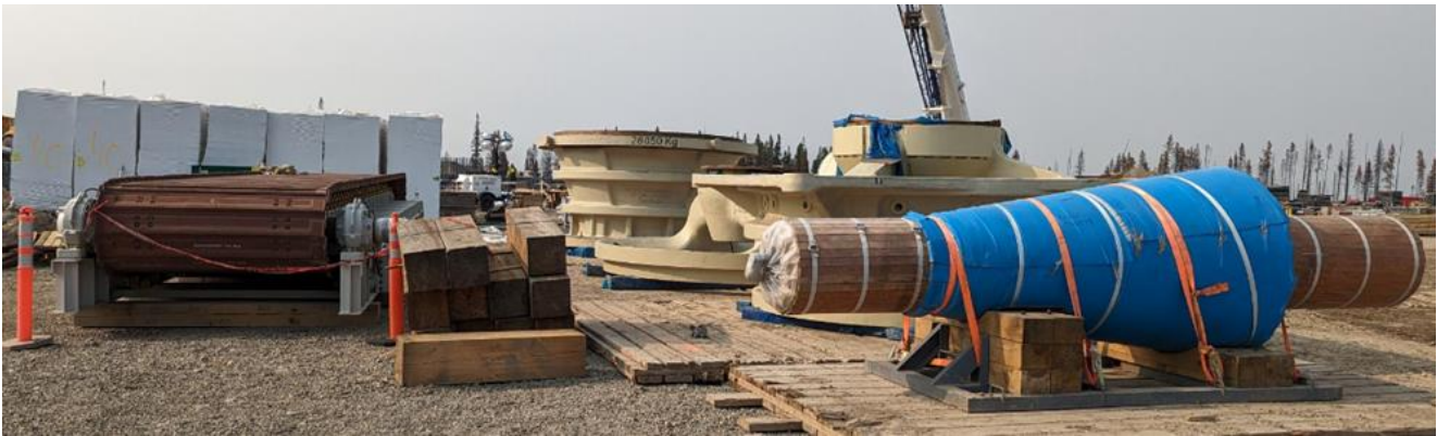
Apron feeder and primary gyratory crusher
