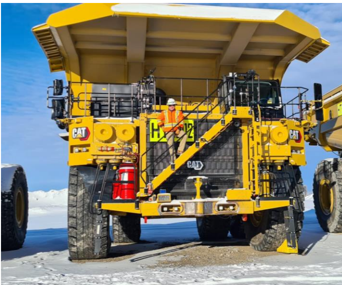
240 Tonne Rigid Frame Haul Truck - January 2024
